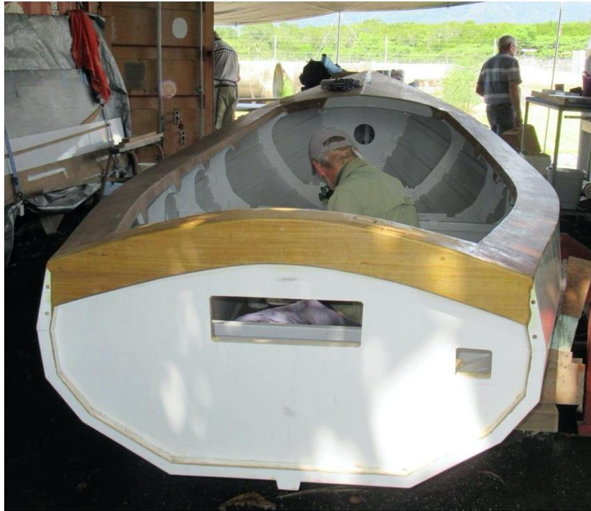
Roger's 15' strip planked canoe is hull-complete with some bracing ribs installed, and other ribs & seat frames being laminated. She will be a thing of beauty once completed – also this year! We have been busy!
